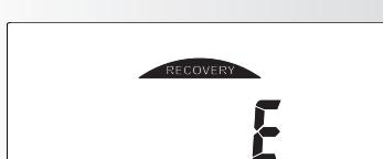
If no pulse is measured in the beginning or at the end of the reverse counting, the error message "E" is displayed
